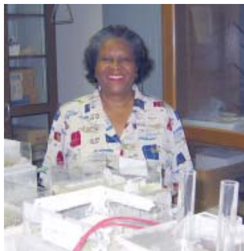
Harovel Wheat among samples of steel and other reinforcements within concrete blocks. The Lucite® boxes constructed atop the concrete blocks allow controlled application of corrosives for testing.
